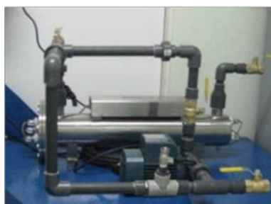
Fig. 1. Photoreactor of NanoTiO 2 /UV air For 60,00 L of water/day
